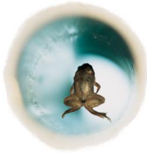
Figure 32-13 An overhead view of a frog that is being levitated in a magnetic field produced by current in a vertical solenoid below the frog. (Courtesy A. K. Gein, High Field Magnet Laboratory, University of Nijmegen, The Netherlands)
