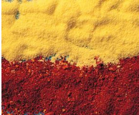
Figure 39-10 Two samples of powdered cadmium selenide, a semiconductor, differing only in the size of their granules. Each granule serves as an electron trap. The lower sample has the larger granules and consequently the smaller spacing between energy levels and the lower photon energy threshold for the absorption of light. Light not absorbed is scattered, causing the sample to scatter light of greater wavelength and appear red. The upper sample, because of its smaller granules, and consequently its larger level spacing and its larger energy threshold for absorption, appears yellow. (From Scientific American, January 1993, page 122. Reproduced with permission of Michael Steigerwald, Bell Labs-Lucent Technologies)
