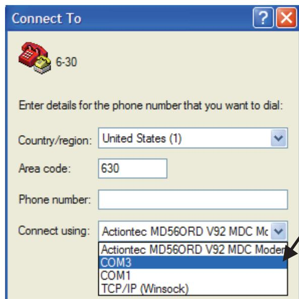
Choose the COM port that the DAQ board is plugged into on the back of your computer (Serial port is COM1 and USB is COM3 for this computer.) COM3, the USB port, is selected here.
